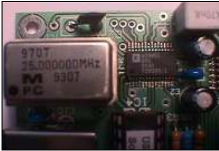
Figure 1. The module with an AD9851 IC and a 25 MHz crystal oscillator.
