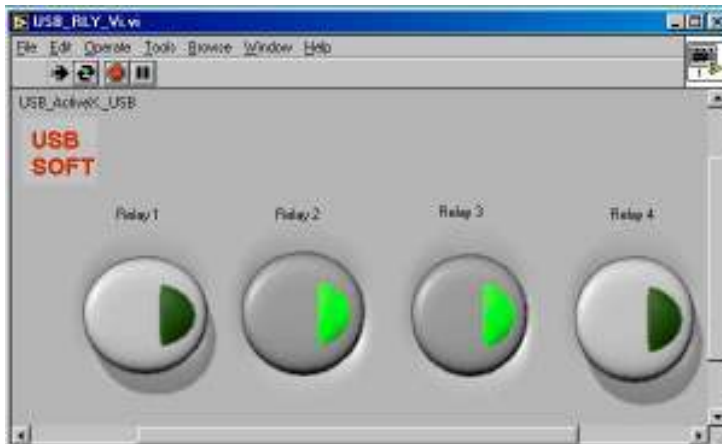
Figure 8. Main vi form. With the USB.OCX, you can control 4 relays on the USB Relay Card.
